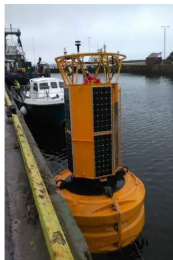
Figure 21. The next generation weather buoy in Galway harbour awaiting deployment on an extended offshore test.
